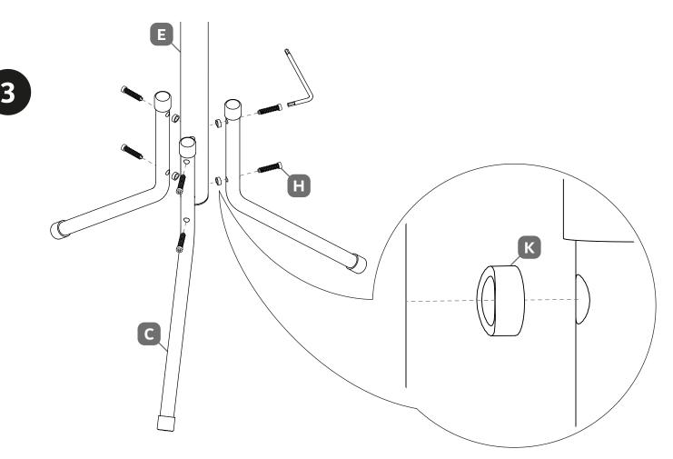
Screw the lower foot pipe to the lower frame pipe.
