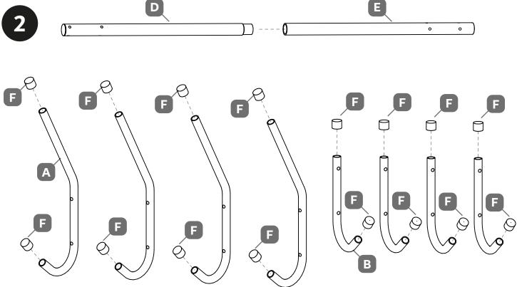
Insert the upper frame pipe to the lower frame pipe and install the small footstand to the upper hanger pipe and middle hanger pipe.
