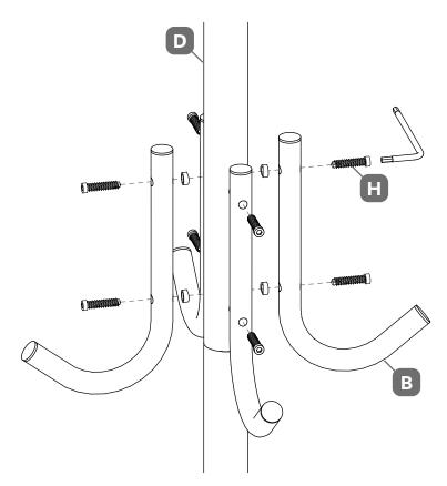
Screw the middle hanger pipe to the upper frame pipe.
