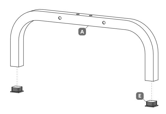
Insert the foot pads into the underframe.
