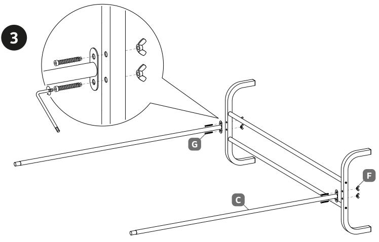
Screw the vertical tubes to the underframes using long screw and butterfly nuts.
