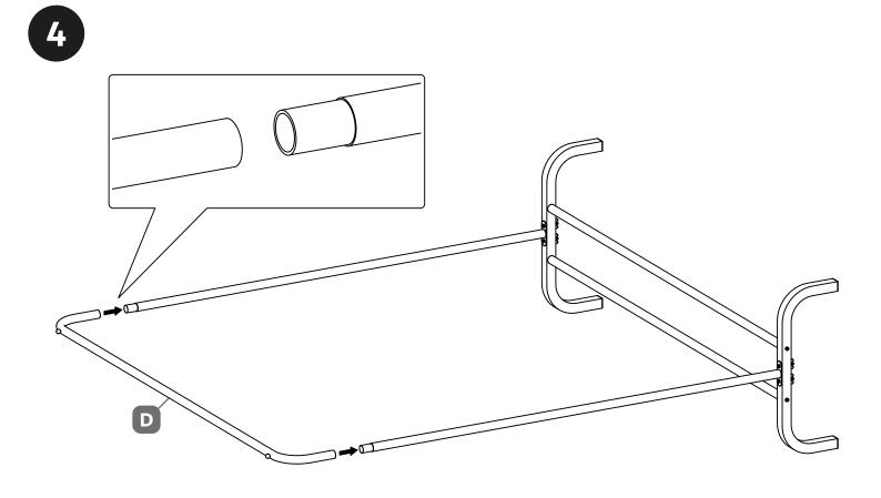
Install the top steel tube to the vertical tubes.
