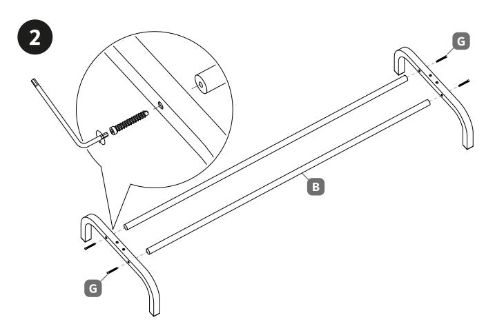
Screw the horizontal tubes to the underframe.
