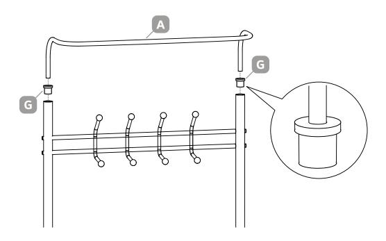
Install the under frame using the connectors.
