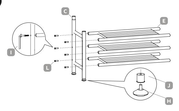
Install left foot frame to the net layers using the long screws.
