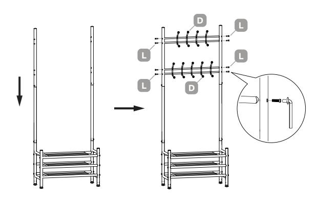
Insert the upper frame pipes to the middle frame pipes and install the hangers to the frame pipes using the long screws then tighten the srews.
