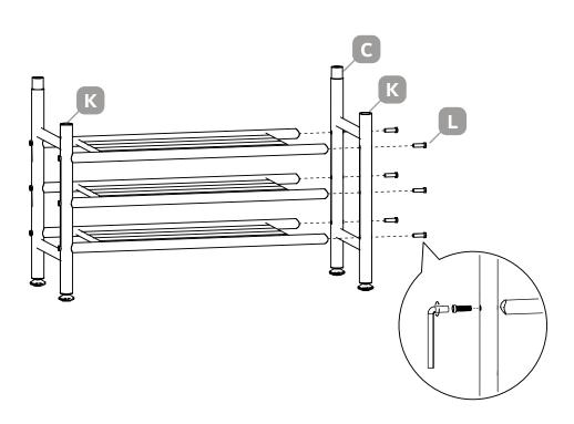
Install left and right foot frames to the net layers using the long screws. Tighten the screws.
