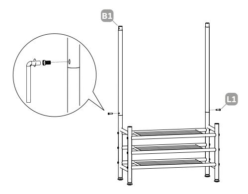
Insert middle frame pipes to the foot frames using the short screws. Tighten the screws.
